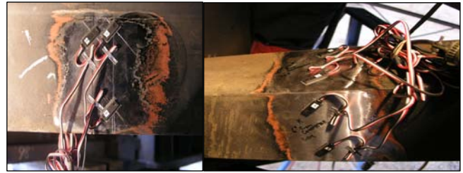
Figure 5. Bending and Axial Circuits at 1/2 Span (left), Bending Strain at 1/4 Span (right)
