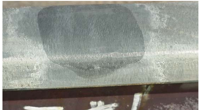
Figure 3. Completed Slot Weld (etched to enhance visibility)
