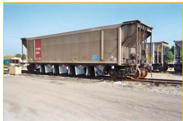
Figure 3: Southern Power's Autoflood Coal Hopper
