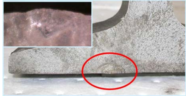
Figure 1. (Circled in red) One of Three Base Fractures. (Upper Left) Plastic Deformation at the Bottom of the Base due to Interaction with the Edge of the Tie Plate.
