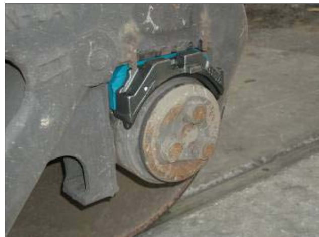
Figure 1: Elastomeric Pedestal Pad in GRL M-976-type Suspension
