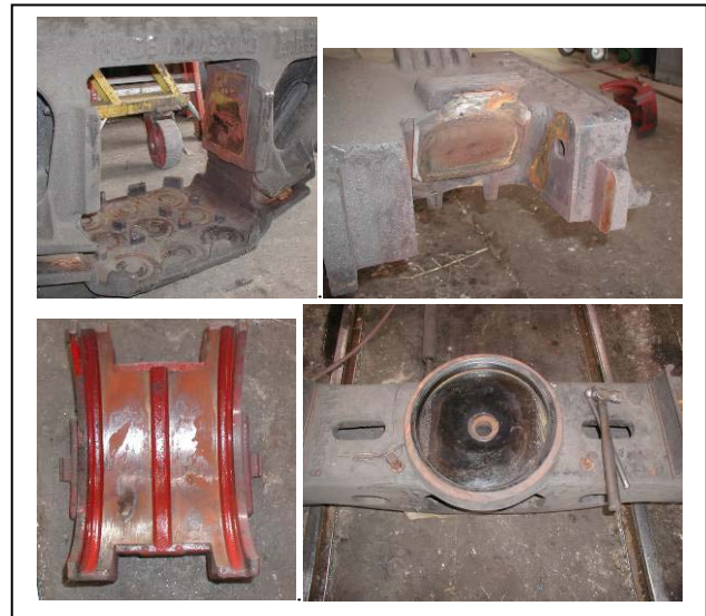
Figure 4: Condition of Lightweight Truck Components after 55,000 Miles
