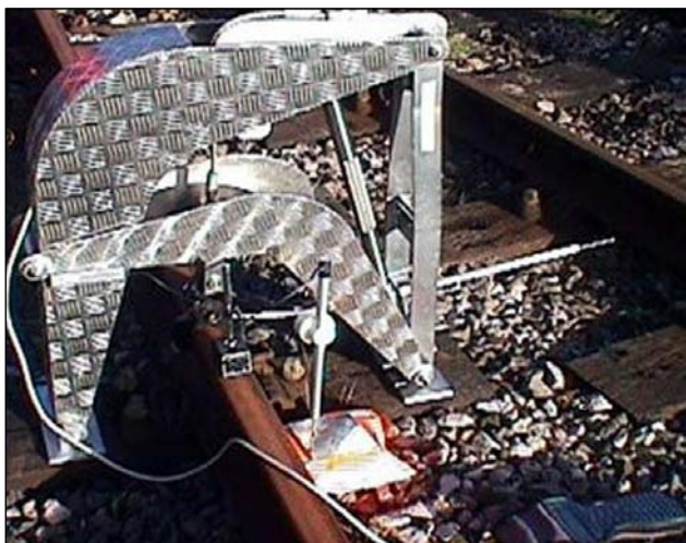
Figure 1. VERSE® Rail Uplift Measurement Hardware
