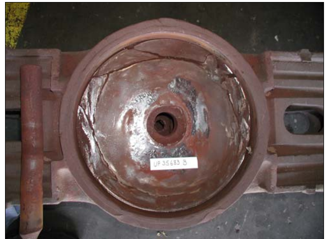
Figure 2. Example of Cracked Center-Plate Liner
