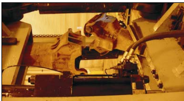
Figure 1. Test Rig used to Test Knuckles at Norfolk Southern
