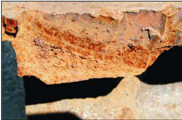
Figure 7. Surface Inclusions from a Knuckle that Experienced Premature Fatigue Failure
