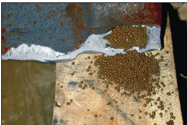
Figure 3. Void in Knuckle Casting Filled with Shot Peen
