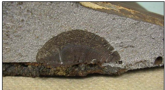
Figure 2: Fatigue fracture of 3/16-inch vertically offset thermite test weld, which initiated at the base of the rail immediately above the flashing intentionally produced for the test (run-out).
