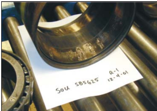
Figure 1. Multiple Cup Spalls
