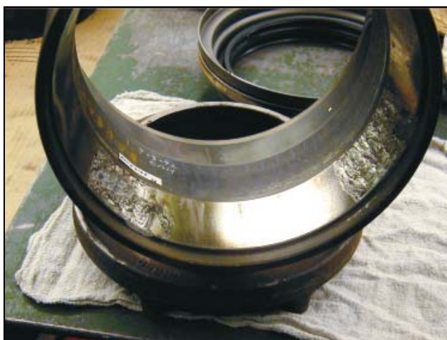
Figure 2. Large Cup Spalling
