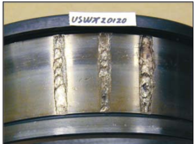
Figure 3. Cone Barline Spalls
