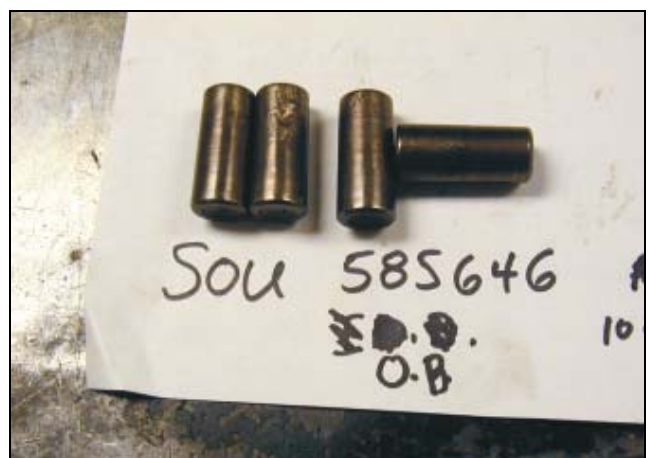
Figure 5. Multiple Roller Spalls
