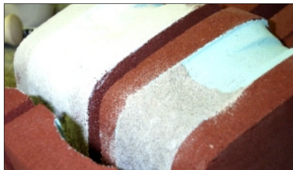
Figure 2. Modifications to a Standard Thermite Weld Mold to Reduce Weld-Toe Flank Angle and Increase Weld Toe Radius (mold modified using refractory cement)
