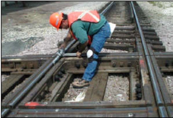
Figure 6. TTCI Measurements of Running Surface Elevation
