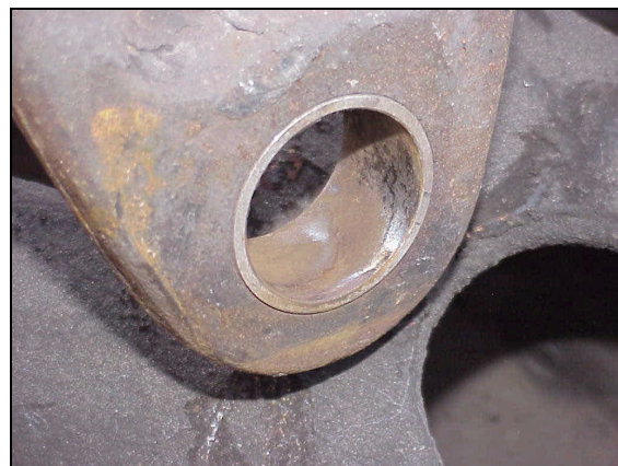
Figure 4. Bushed Brake Beam Live Lever from Car 97542.
