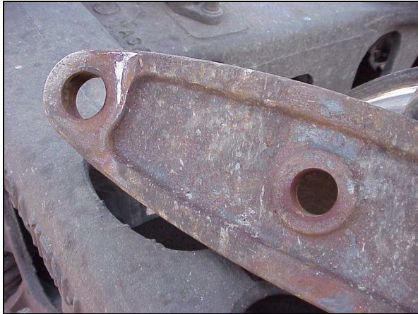
Figure 5. Live Truck Lever showing almost no wear after 240,000 miles — Car 97405
