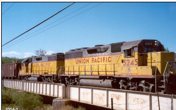
Figure 4. Three-Span TPG Test Bridge on UP at Adobe, Colorado
