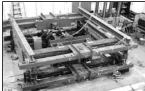
Figure 2. Fatigue Loading Frame
