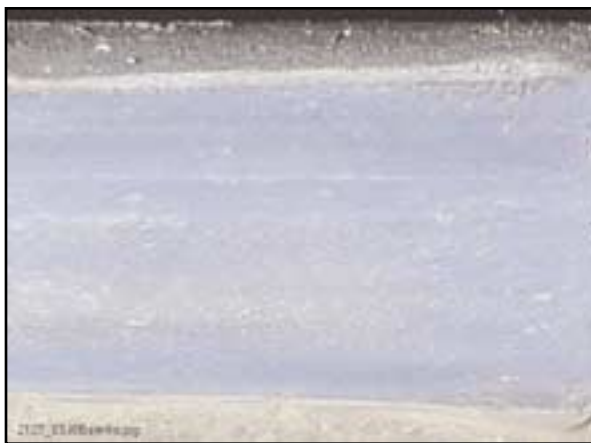
Exhibit 3. J6 Bainitic Rail from the Inside of the Curve (low rail) Shows No Evidence of Rolling Contact Fatigue on the Rail Surface Rail surface shown at 110 MGT
