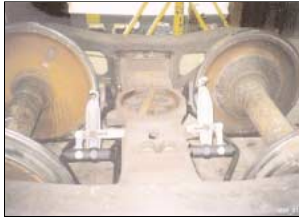
Exhibit 1. Link Support System Installed on the FAST Car
