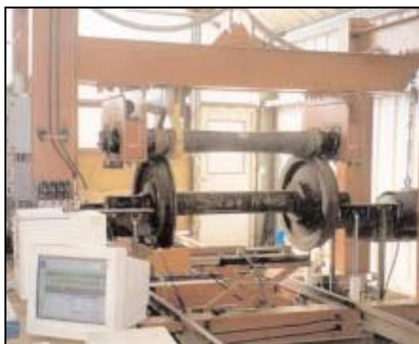
Exhibit 2. Shop Trial UT System Set Up
