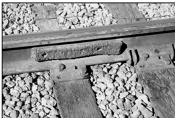
Exhibit 5. Heat Damaged Strain Gage Sensor Cover
