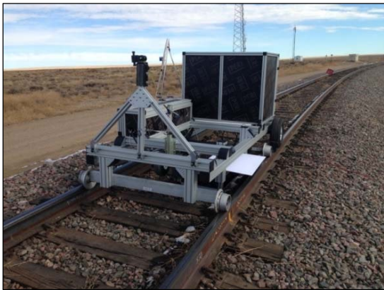
Figure 5: Prototype Rail Stress Measurement System Cart
